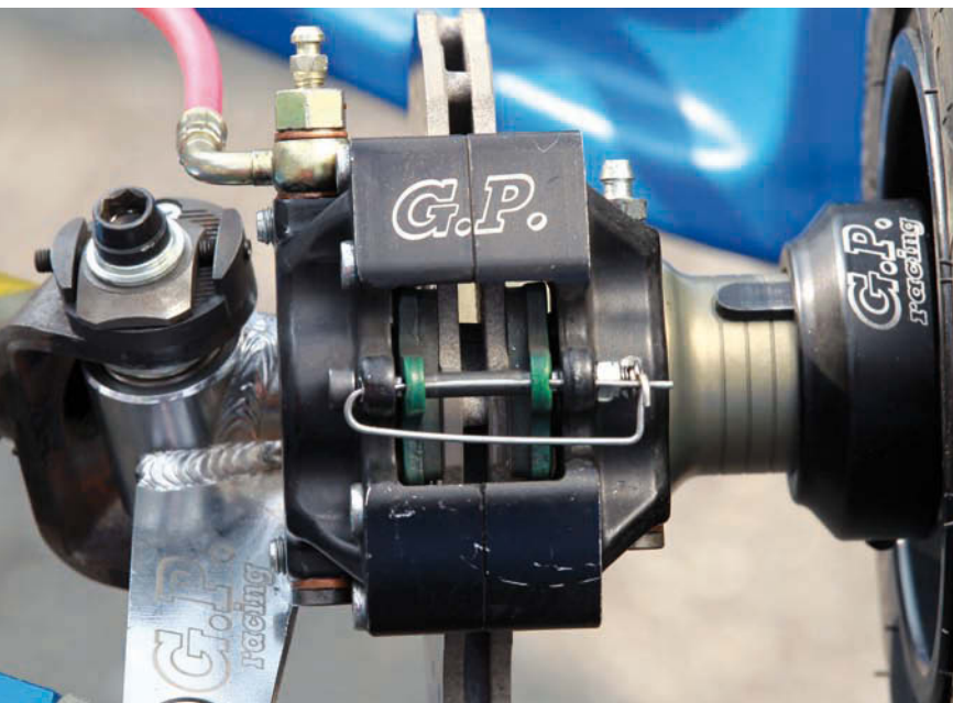
"Cams" (so to speak) made by Sniper are used to adjust fore-carriage, while the braking system is the optional one with discs made of ceramic material, Duralcam. Always on request there are magnesium components instead of the aluminium one and "manual" front brakes for KF2.
